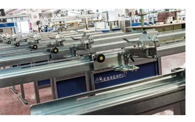
The "Messerfix" is a universal sharpening tool for all common mowing blades and hedge trimmers. With this sharpening tool, sharpening mowing blades becomes easy for everyone. The mowing blade is clamped in place comfortably using the adjustable holders and does not need to be re-clamped during the sharpening process.
